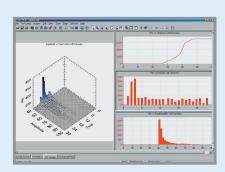
**Above**: AEwin's 3-D graphing capability allows the graph to be rotated freely, using the mouse. **Below**: A typical activity screen with both AE features and waveforms, processed with a simple mouse clickz for any specific hit.
